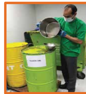
Filtering waste oil
